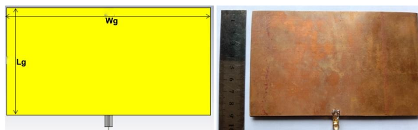
Figure 2. Microstrip antenna circular patch (back view).
