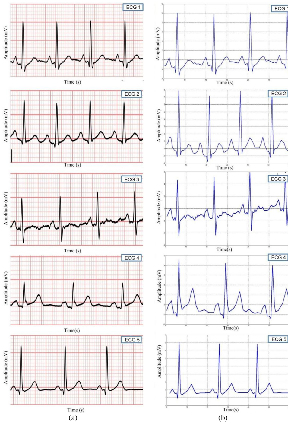
Figure 3. (a) ECG signal data 1 – 5 displayed on standard ECG paper, (b) The result of converting numerical data into heart rhythm from ECG 1 – 5 using MATLAB.
