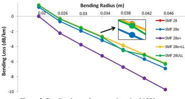
Figure 2. Bending losses for a wavelength of 1550 nm.
