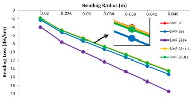
Figure 1. Bending losses for wavelength 1310 nm.
