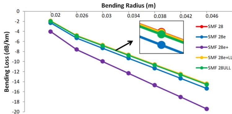
Figure 1. Bending losses for wavelength 1310 nm.
