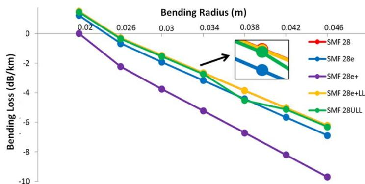
Figure 2. Bending losses for a wavelength of 1550 nm.
