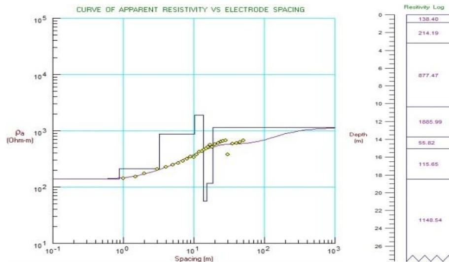
Figure 9. Geoelectric line data graph 4 Schlumberger configuration.
