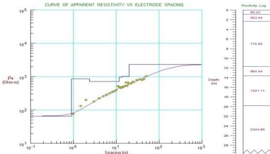
Figure 7. Geoelectric line data graph 2 Schlumberger configuration.
