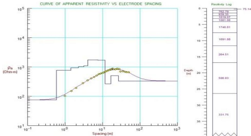
Figure 8. Geoelectric line data graph 3 Schlumberger configuration.
