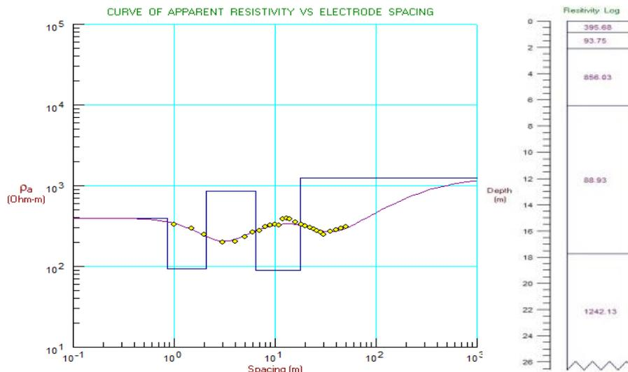
Figure 6. Geoelectric line data graph 1 Schlumberger configuration.
